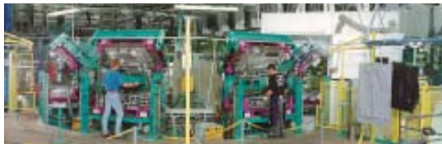
Rotating die-casting equipment of Krauss-Maffei Kunststofftechnik (Munich); in operation at Johnson Control Interiors (Lüneburg)
