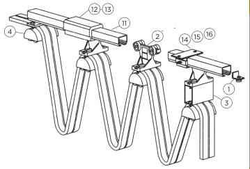
Required Flatcable length = Track length + 10% + 2 Tails @ V = 30m/min Required Roundcable length = Track length + 15% + 2 Tails @ V = 30m/min
